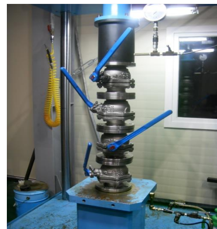
BALL VALVE HYDROSTATIC TEST
