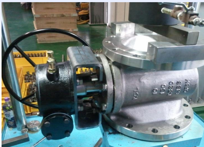
PLUG VALVE HYDROSTATIC TEST
