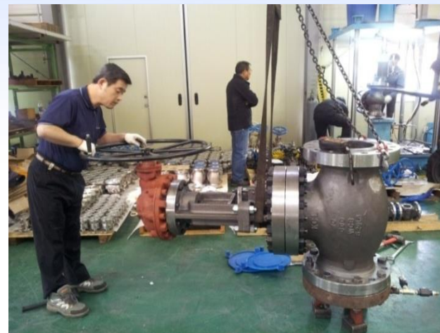
600LB GLOBE VALVE FUNCTIONING TEST
