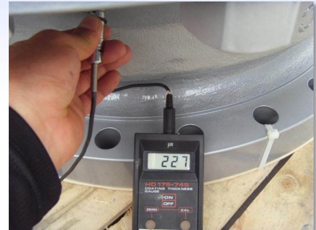
Paint Thickness TEST
