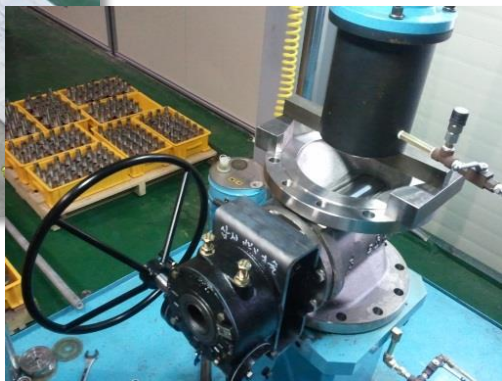
600LB GLOBE VALVE FUNCTIONING TEST
